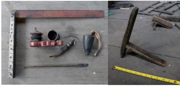
Figure 10. Tools used for the mark-ink work (left). Douchi (right).
